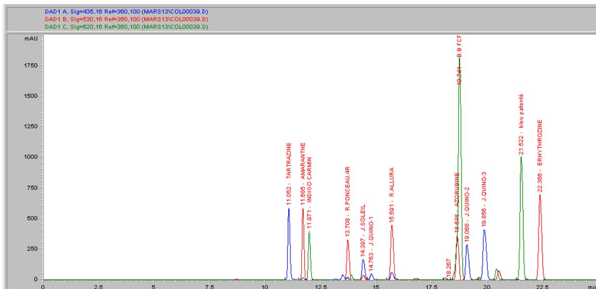
Figure 2: Chromatogram of a mixed standard solution of 11 dyes.
